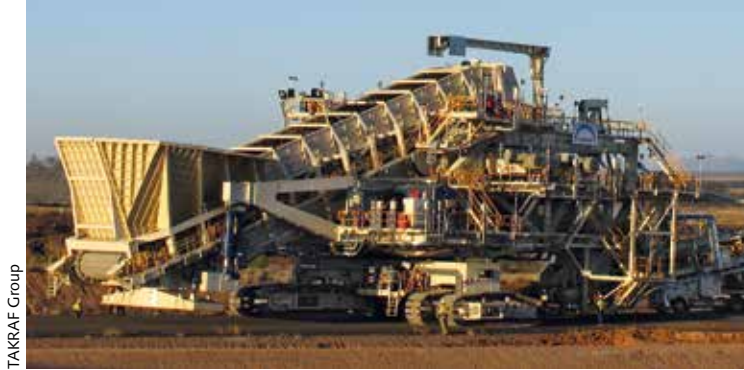
12,000 t/h mobile Brechanlage in Australien 12,000 t/h mobile crushing plant in Australia
